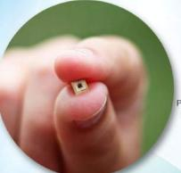
Mercury Free Conventional UV lamps contain mercury, but UV LEDs are free of hazardous materials which eliminates risk of mercury spill due
